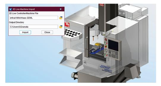
The 3DLive Interface reads in 3D Geometry for CNC machines, fixtures and cutting tool holders, including:
